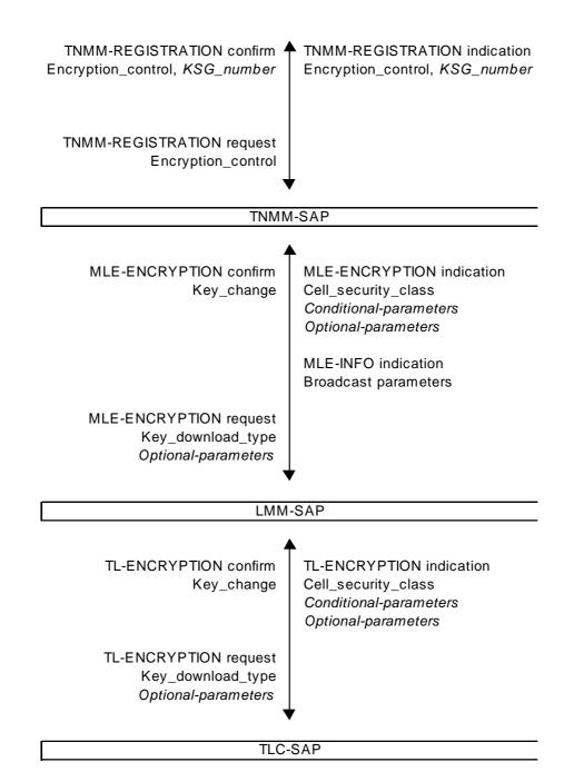
Figure 6.14: Protocol stack and primitives for encryption control
