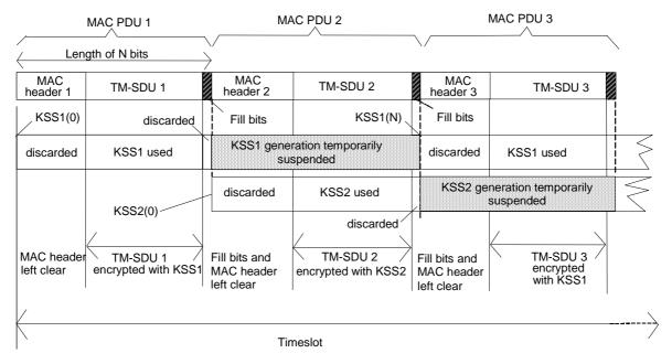
NOTE: In this example, TM-SDU 1 and TM-SDU 3 use the same DCK but TM-SDU 2 uses a different DCK.
