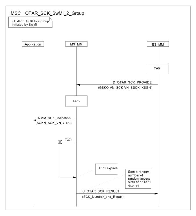
NOTE: Although SCK is sealed by the group key the D-OTAR SCK PROVIDE may be distributed to either a group or an individual address and encrypted appropriately.
