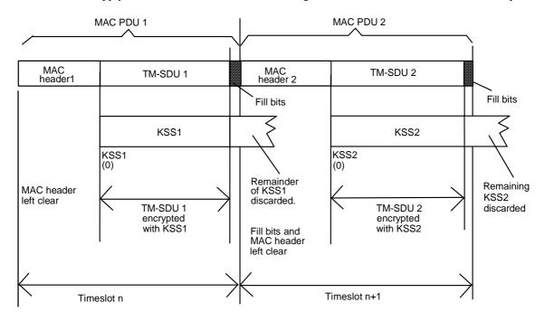
Figure 6.3: Allocation of KSS to encrypt MAC PDUs
