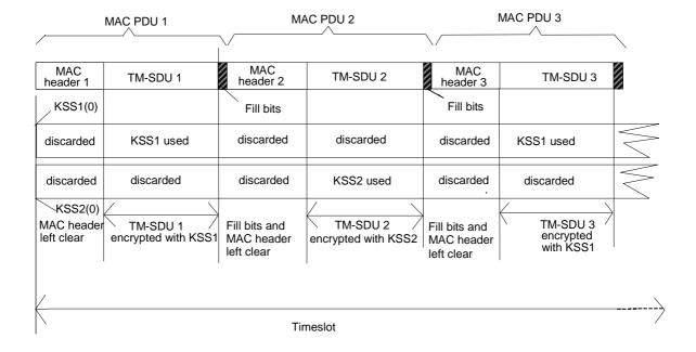
NOTE: In this example, TM-SDU 1 and TM-SDU 3 use the same cipher key but TM-SDU 2 uses a different cipher key.
