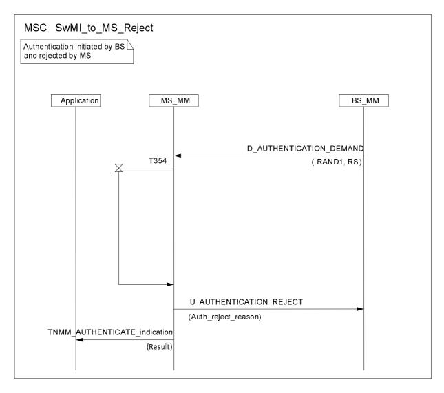
Figure 4.25: Authentication initiated by SwMI and rejected by MS
