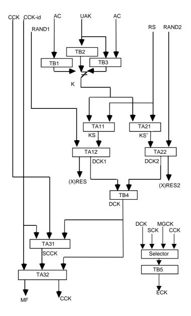
NOTE: Algorithms TB1, TB2 and TB3 are shown for information and may be used in deriving K within an MS.
