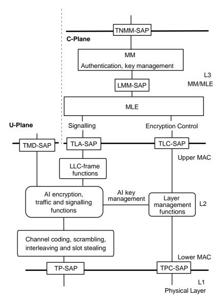
Figure 6.1: Relationship of security functions to layers functions in MS
