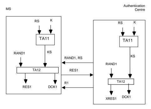
Figure 4.1: Authentication of a MS by the infrastructure
