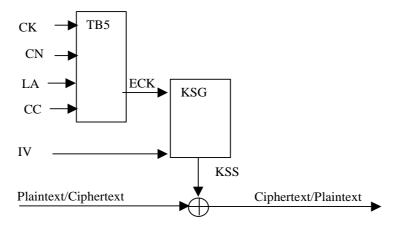
NOTE: CN of the main carrier, CC, LA-id, and initializing values of IV are received at the MS from the BS broadcast signalling messages. After initialization IV is locally generated at the MS. When camped on a cell CN values are received at the MS from downlink MAC-RESOURCE and MAC-END PDUs. IV is locally generated at the BS.
