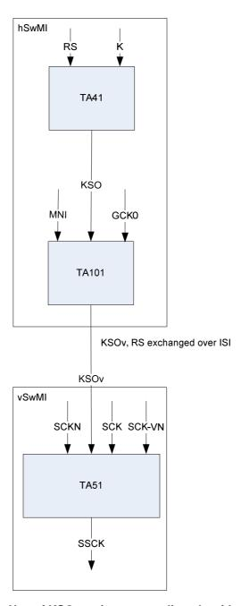
Figure 4.49: Use of KSOv as input to sealing algorithm TA51 in vSwMI
