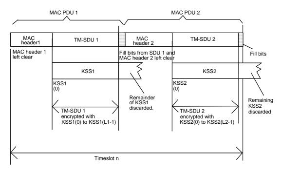
NOTE: Length of TM-SDU 1 is L1, length of TM-SDU 2 is L2.
