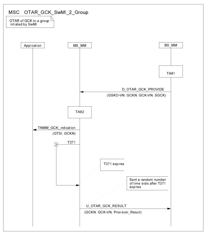
NOTE: Although GCK is sealed by the group key the D-OTAR GCK PROVIDE may be distributed to either a group or an individual address and encrypted appropriately.
