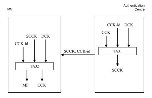
Figure 4.10: Distribution of a common cipher key
