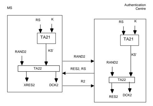
Figure 4.2: Authentication of the infrastructure by a MS
