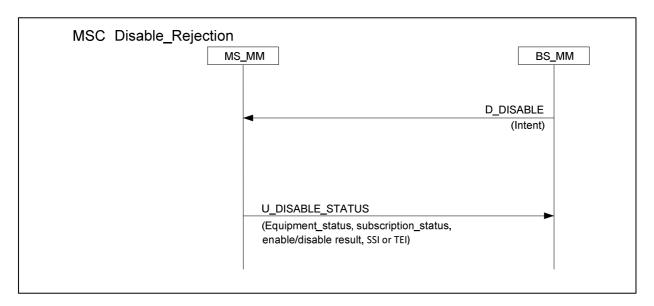
Figure 5.9: Rejection of permanent disabling by an MS without authentication
